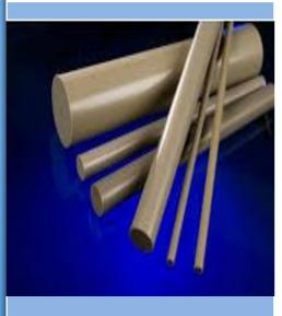
PEEK (Ploy Ether Ketone) is a high performance engineering thermoplastic that offers chemical and water resistance similar to PPS, but can operate at higher temperatures. PEEK can be used continuously to 480° F (250°C) and in hot water or steam without permanent loss in a physical properties. For hostline environments, PEEK is high stength alternative to fluoropolymers. PEEK Carres a V-0 flammability rating and exhibits very low smoke and toxic gas emission when exposed to flame.
