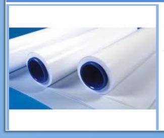
Standard Size: 300 x 300 mm, 450 x 450 mm, 600 x 600 mm, 1000 x 1000 mm, 1200 x 1200 mm, 1500 x 1500 mm, 1000 x 2000 mm, 2000 x 2000 mm. Thickness: 0.1 mm to 5.0 mm(Standard). Made to Order: Specific Length, Width & Thickness available for customer's requirement. Filler : Glass / Carbon / Graphite /Bronze / Bronze + Mos<sub>2</sub> Material : Virgin PTFE & Filled PTFE.
