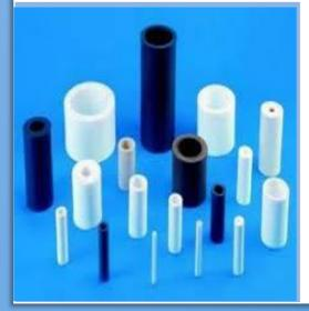
Outer Diameter : 12.5 mm to 300 mm (Standard). Inner Diameter : 6mm to 275mm (Standard). Length : 100 mm (Standard) Made to Order: Specific O.D. & I.D. available as per customer's requirement. Filler : Glass / Carbon / Graphite / Bronze + Mos2. Material : Virgin PTFE & Filled PTFE. Specification No. : ASTM - D 3295.
